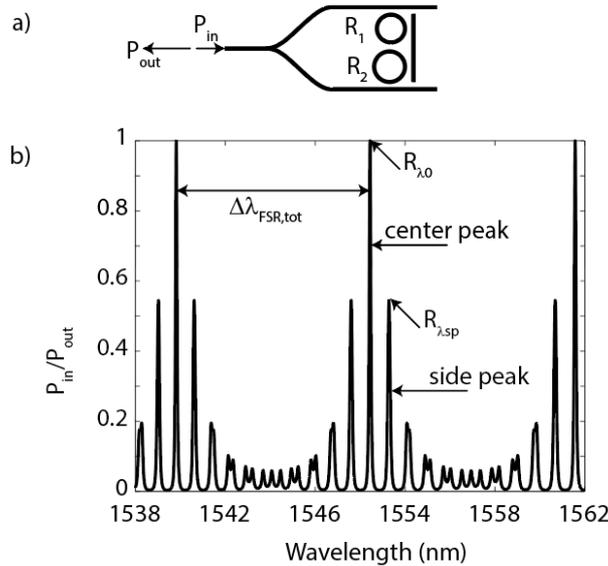
Figure 2. a) Schematic layout of a ring resonator mirror with two differently sized rings with  $R_1$  and  $R_2$  radii. b) Reflected power vs. input wavelength calculated for a ring resonator with an FSR of about 1.6 nm, while the second ring has a 10% larger radius.
