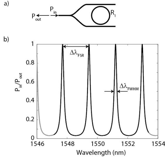
Figure 1. Schematic layout of a ring resonator mirror with a single ring resonator with radius  $R_1$ . (b) Reflected power vs. input wavelength calculated for a ring resonator with an FSR of about 1.6 nm.
