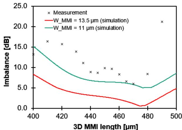
Figure 12: Imbalance as a function of the 3D MMI length for measurement (crosses) and simulation (red and green line) for a waveguide width of  $3.5\ \mu\text{m}$  and horizontal waveguide distance of  $9.0\ \mu\text{m}$ . The measurement results are obtained from structures with a nominal 3D MMI width of  $13.5\ \mu\text{m}$ .
