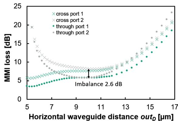
Figure 6: Simulated loss at 1550 nm as a function of the horizontal waveguide distance of a 3D 4x4 MMI for a fixed 3D MMI length of  $450 \mu\text{m}$ , 3D MMI width of  $13.5 \mu\text{m}$  and a waveguide width of  $3.5 \mu\text{m}$ .
