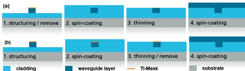
Figure 9: Schematic sketches of the fabrication process sequence of a 3D MMI for the standard process (a) [9] and the optimized process (b) [5].
