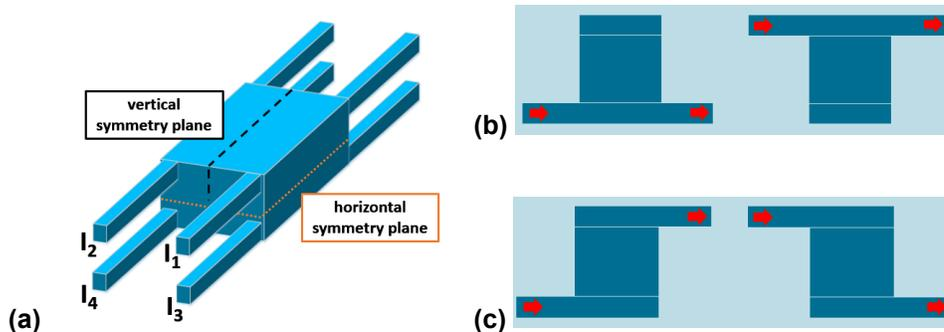
Figure 4: Sketch of the symmetry planes on a 3D 4x4 MMI. (a) Overview of a 3D 4x4 MMI with the horizontal and vertical symmetry plane. Grouped connection modes in (b) ‘through’ and (c) ‘cross’ shown in the longitudinal section of a 3D 4x4 MMI.
