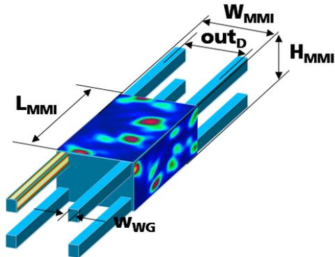
Figure 2: 3D sketch of a 3D 4x4 MMI with simulation results for the light intensity.
