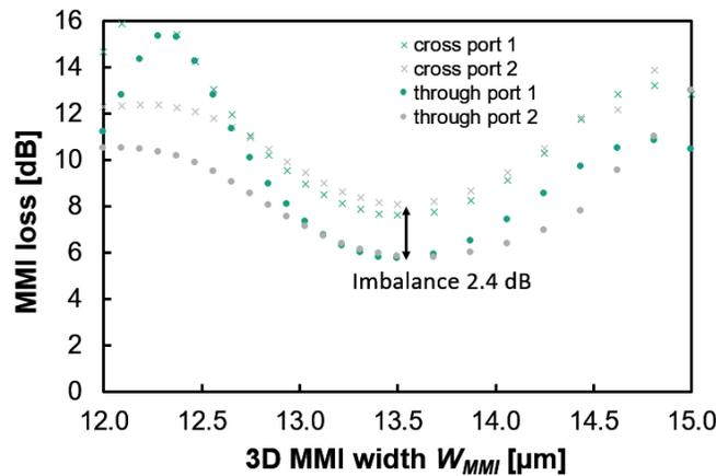
Figure 5: Simulated loss at 1550 nm as a function of the 3D 4x4 MMI width for a fixed 3D MMI length of  $450 \mu\text{m}$ , a waveguide width of  $3.2 \mu\text{m}$ . The horizontal waveguide distance changed with the 3D MMI width.
