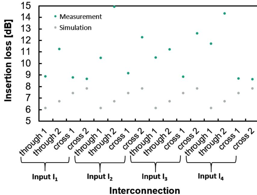
Figure 11: Measured and simulated insertion losses for each interconnection of a 3D 4x4 MMI (length of 470  $\mu\text{m}$ , width of 13.5  $\mu\text{m}$ , waveguide width of 3.5  $\mu\text{m}$ , horizontal waveguide distance of 9.0  $\mu\text{m}$  and includes 1.2 dB: material absorption, fiber-chip-fiber coupling loss; loss determined with straight reference waveguides) at a wavelength of 1550 nm.
