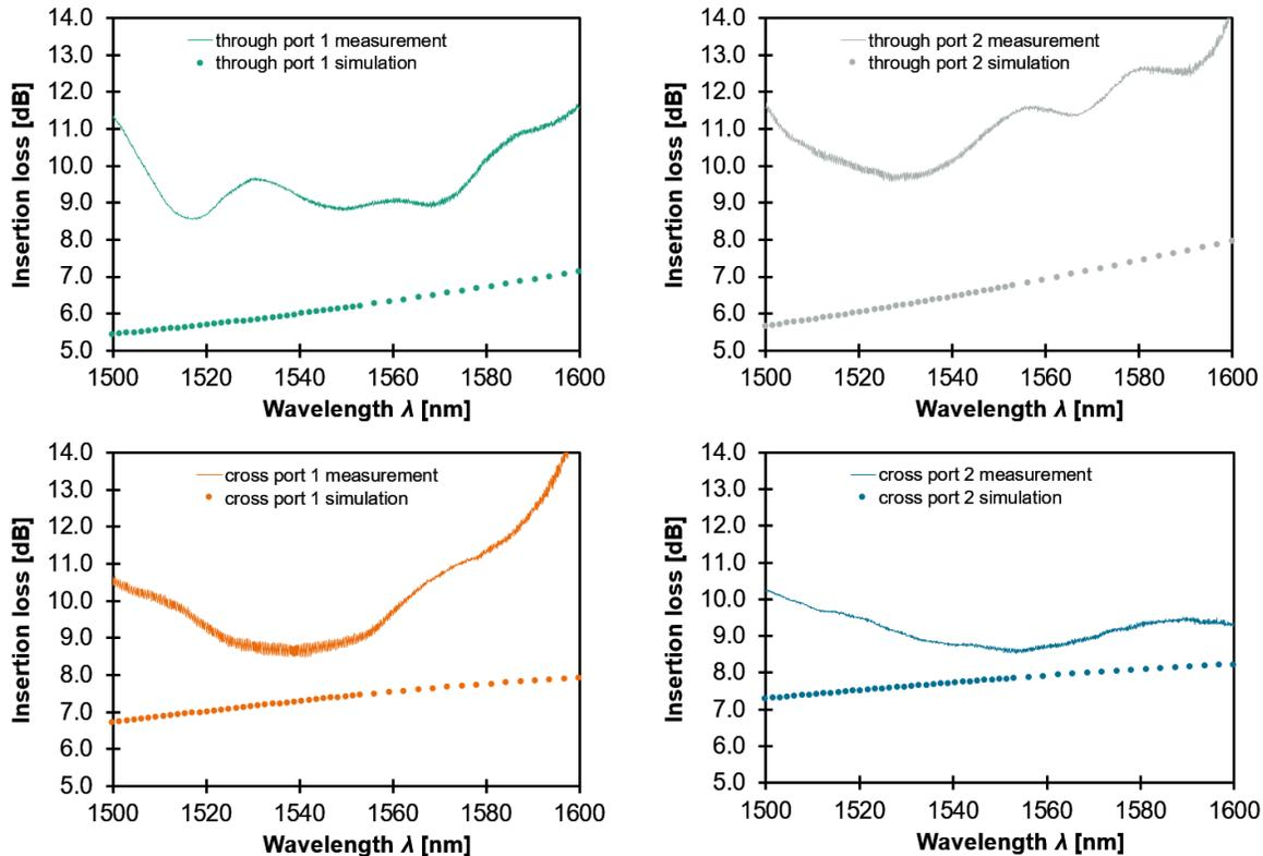
Figure 10: Optical transmission measurements on a 3D 4x4 MMI for one input  $I_1$  with all connection modes for a 3D MMI length of  $470 \mu\text{m}$ , width of  $13.5 \mu\text{m}$ , waveguide width of  $3.5 \mu\text{m}$  and a horizontal waveguide distance of  $9.0 \mu\text{m}$  (includes 1.2 dB: material absorption, fiber-chip-fiber coupling loss; loss determined with straight reference waveguides). Additionally, for each connection the simulation results for the given parameters are shown.
