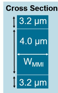
Figure 3: Schematic of the cross section of the 3D 4x4 MMI section with three waveguide layers.
