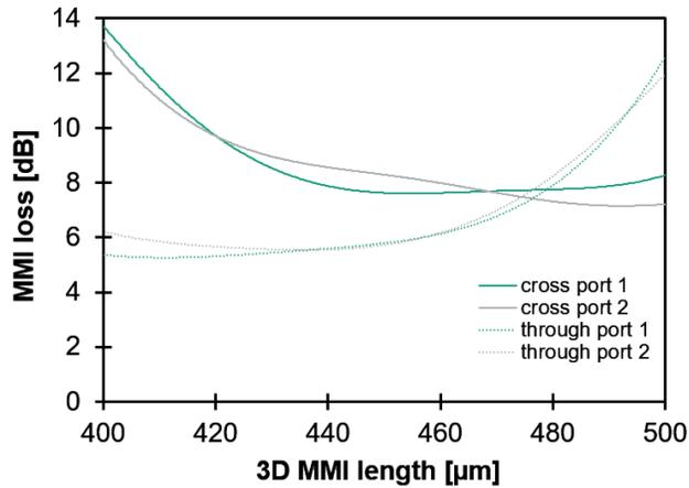
Figure 7: Simulated loss at 1550 nm as a function of the 3D MMI length for a fixed 3D MMI width of 13.5  $\mu\text{m}$ , waveguide width of 3.5  $\mu\text{m}$  and horizontal waveguide distance of 9.6  $\mu\text{m}$ .
