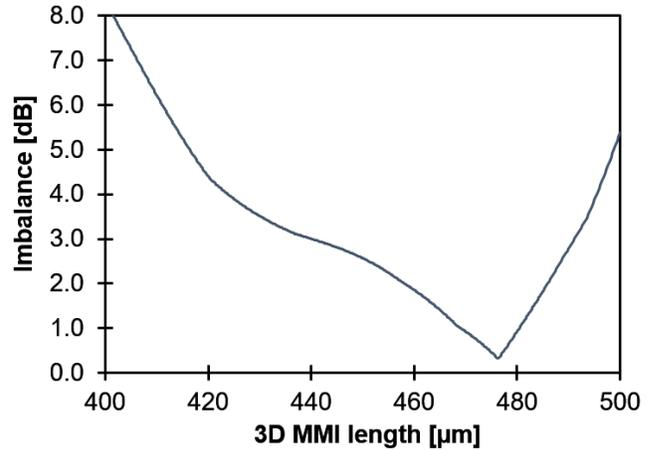
Figure 8: Simulated imbalance at 1550 nm as a function of the 3D MMI length for a fixed 3D MMI width of 13.5  $\mu\text{m}$ , waveguide width of 3.5  $\mu\text{m}$  and horizontal waveguide distance of 9.6  $\mu\text{m}$ .
