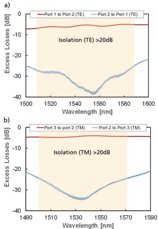
**Fig. 4:** On-chip transmission in forward and backward direction of the fabricated optical isolator, for TE polarization (a) and TM polarization (b).
