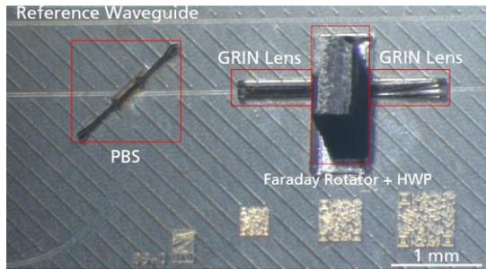
**Fig. 3:** Fabricated optical isolator with highlighted integrated micro optical elements.
