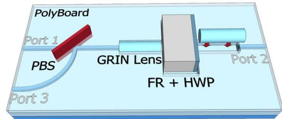
**Fig. 1:** Schematic layout of the optical isolator, consisting of polymer waveguides, an inserted polarizing beam splitter (PBS) and a on-chip free-space region created by two GRIN lenses to integrate a bulk Faraday rotator and a half wave plate.
