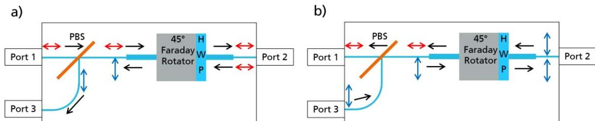
**Fig. 2:** Working principle of the optical isolator for TE polarization (red horizontal arrows) from Port 1 (a) and TM polarization (blue vertical arrows) from Port 3 (b).
