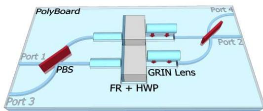
**Fig. 5:** Proposed structure for a polarization-independent optical circulator/isolator (under investigation).
