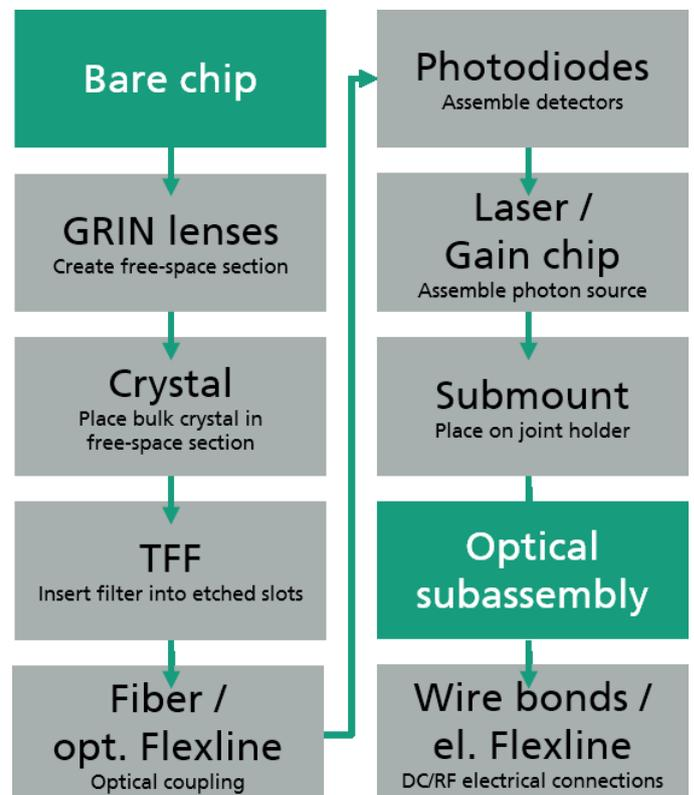
Fig. 5. Generic semi-automated assembly process of a hybrid photonic integrated circuit on the PolyBoard platform.
