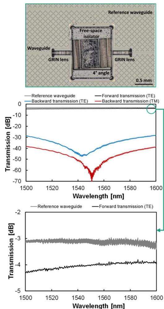
**Fig. 2:** Micrograph of an optical isolator integrated on a polymer-based PIC (top) and measured spectra of forward and backward transmission (middle). Magnification of the forward transmission spectrum (bottom).
