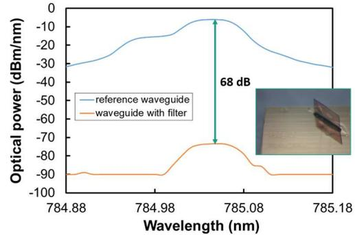
**Fig. 4:** Transmission through a waveguide with TFF for the suppression of 785 nm light compared to a reference waveguide without filter. The inset shows an exemplary PIC with inserted dielectric TFF.
