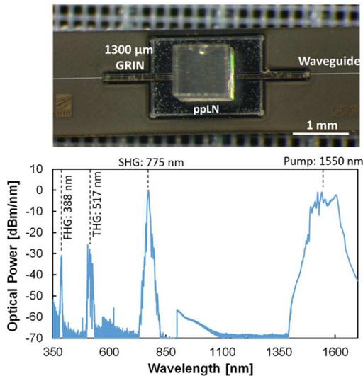
**Fig. 3:** Micrograph of a ppLN crystal integrated on a polymer-based PIC (top) and measured spectra of higher harmonics when pumped with an fs-pulse laser around 1550 nm (bottom) [10].
