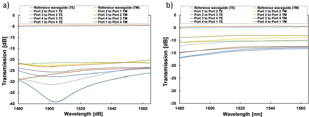
Figure 4. Measured insertion loss, including fiber-chip coupling losses of  $\sim 1.5$  dB per facet, in forward (a) and backward (b) transmission for all ports in TE and TM polarization.
