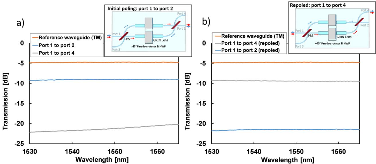
Figure 5. Repoling between the ports enables switching as illustrated in Figure 2 (a) and (c). Here, switching is demonstrated for port 1 as the input port and port 2 and 4 as the output ports. a) Initial poling with transmission from port 1 to port 2 and optical isolation of port 4. b) Repoled Faraday rotators with transmission from port 1 to port 4 and optical isolation of port 2.
