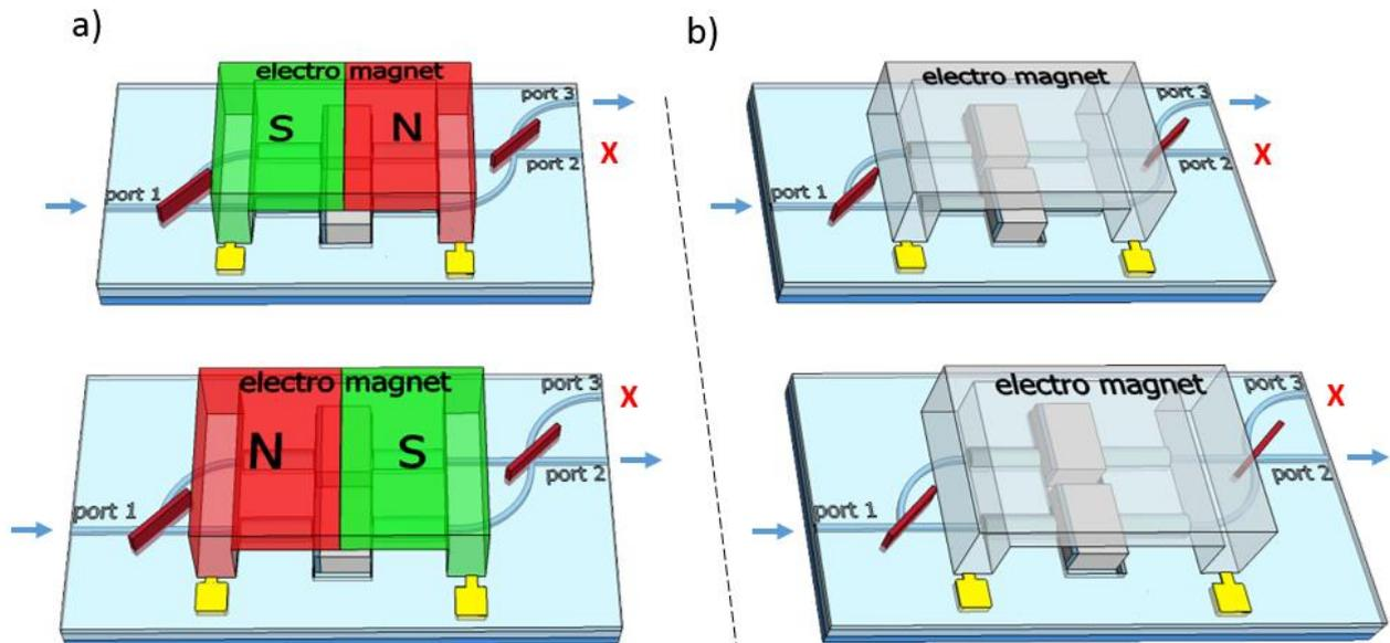
Figure 6. Concept of a latching switch based on the optical circulator with an added electromagnet. Depending on the applied current and magnetic field, the Faraday rotators are poled or repoled (a). After switching off the electro magnet, the Faraday rotators and the circulator maintain their polarization state indefinitely (b).
