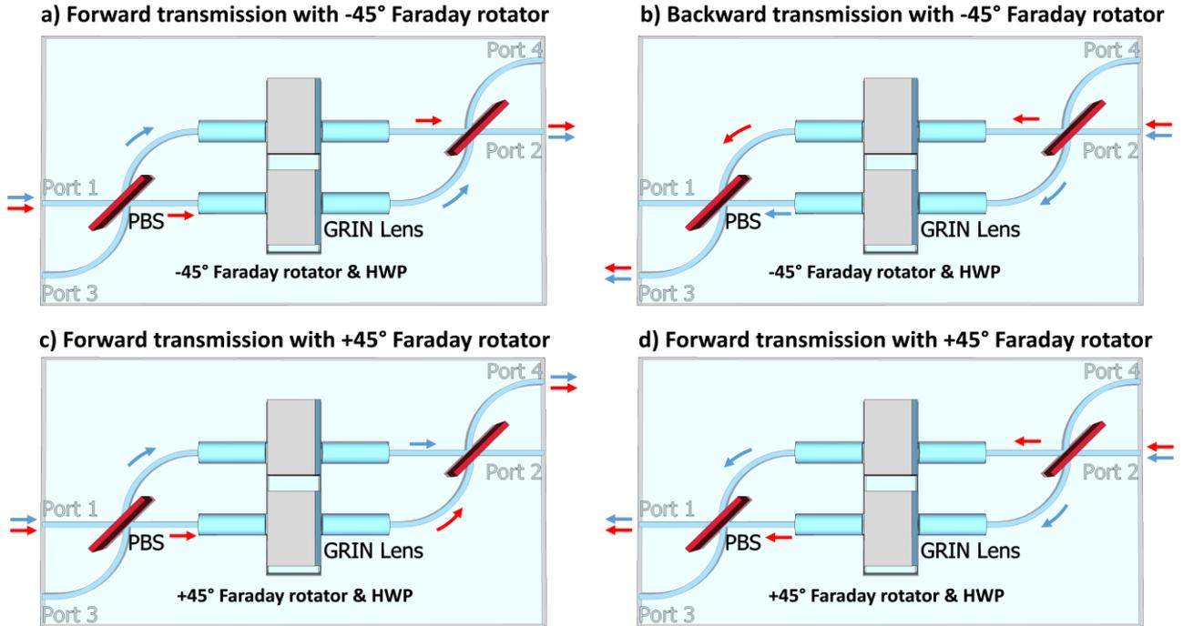
Figure 2. Working principle of the optical circulator in forward and backward transmission for TE (red arrows) and TM (blue arrows) polarized light with a  $-45^\circ$  Faraday rotator (a, b) and a  $+45^\circ$  Faraday rotator (c, d). The output port depends on the magnetization and direction of Faraday rotation of the Faraday rotator.
